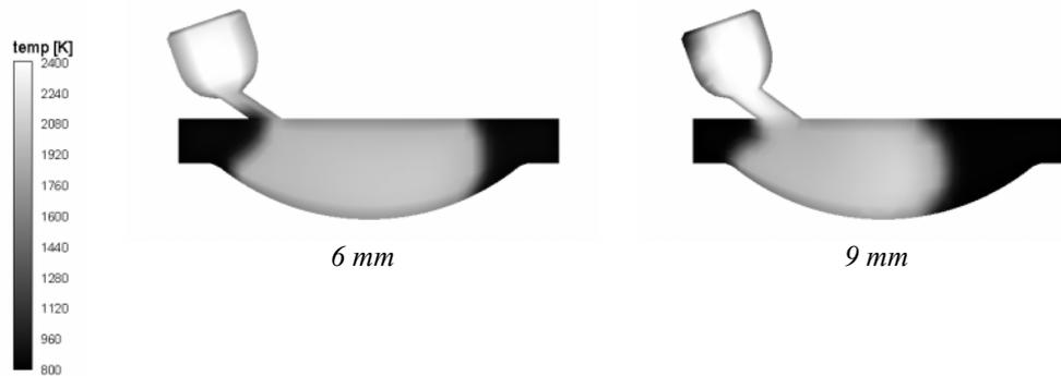
Fig. 10. Temperature distribution in combustion chambers of modeled engine for  $\lambda = 2.0$  at  $5^\circ\text{CA}$  after TDC
