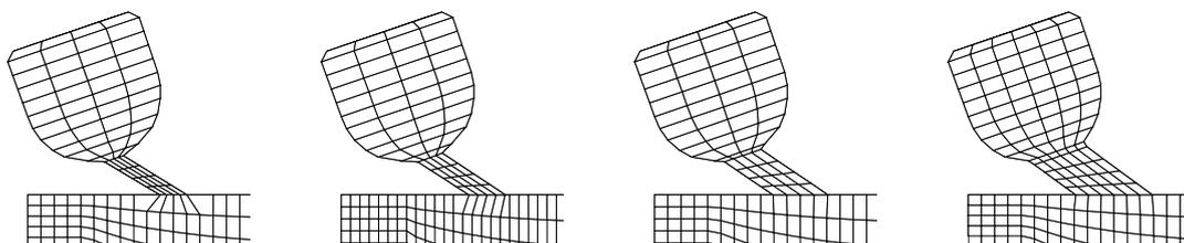
Fig. 2. Parts of geometric mesh with connecting duct of diameter equal: 3mm, 4 mm, 6 mm, 9 mm
