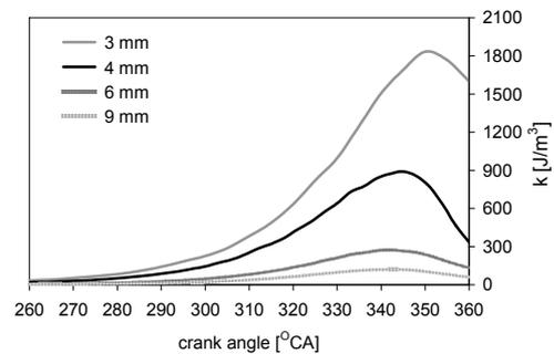
Fig. 4. The kinetic energy of turbulence in the prechamber of two-stage combustion system engine
