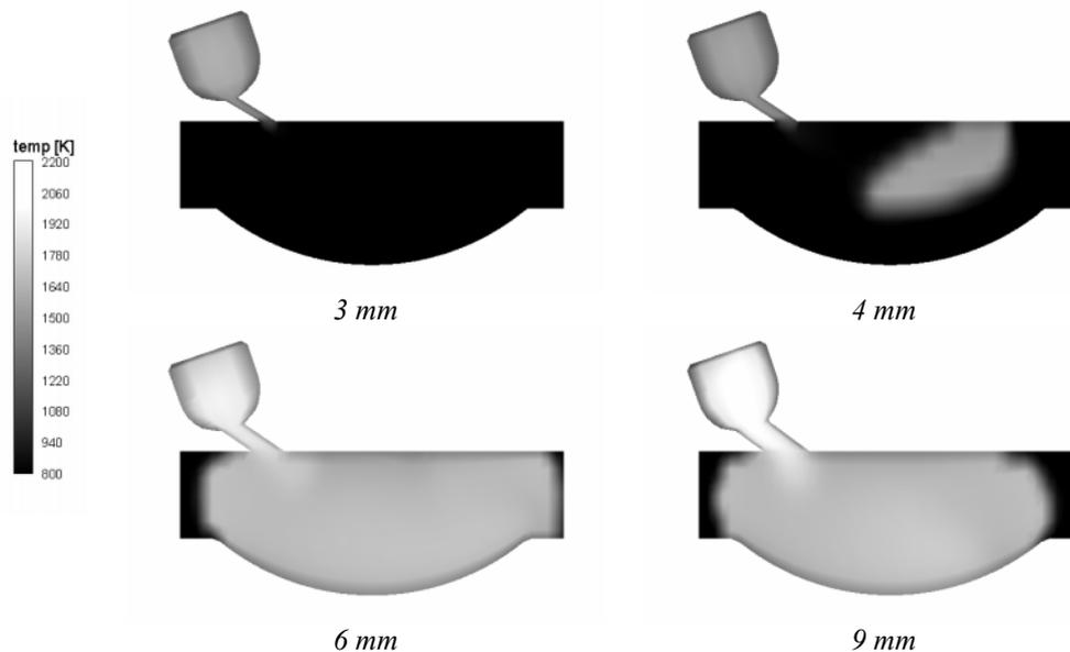
Fig. 10. Temperature distribution in combustion chambers of modeled engine for  $\lambda = 2.0$  at  $30^\circ\text{CA}$  after TDC
