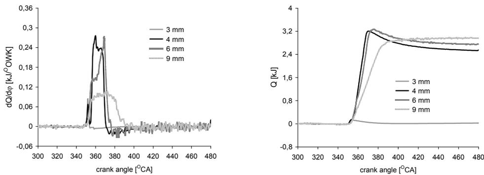
Fig. 12. Heat release rate and amount of heat released during combustion in function of CA for  $\lambda=1.6$
