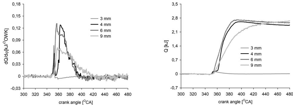
Fig. 13. Heat release rate and amount of heat released during combustion in function of CA for  $\lambda=1.8$
