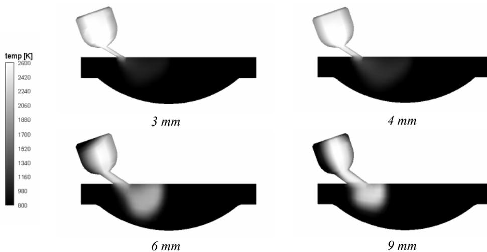
Fig. 10. Temperature distribution in combustion chambers of modeled engine for  $\lambda = 2.0$  at  $5^\circ\text{CA}$  before TDC
