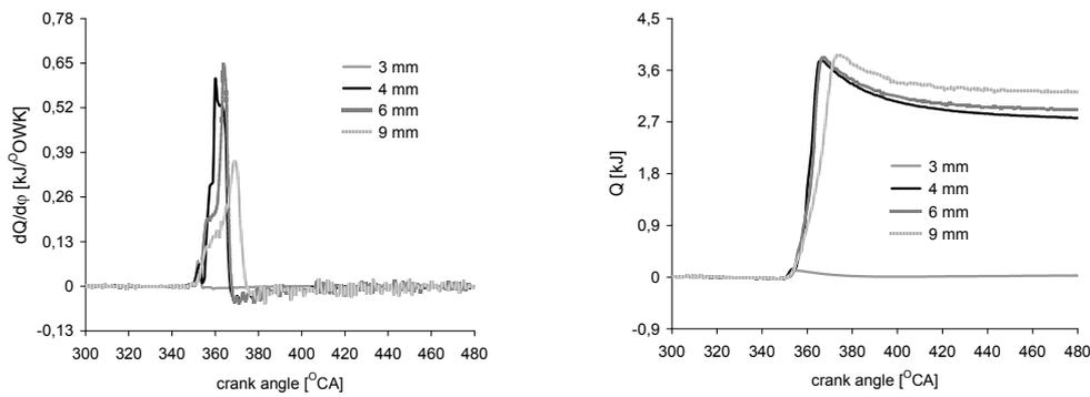
Fig. 11. Heat release rate and amount of heat released during combustion in function of CA for  $\lambda=1.4$
