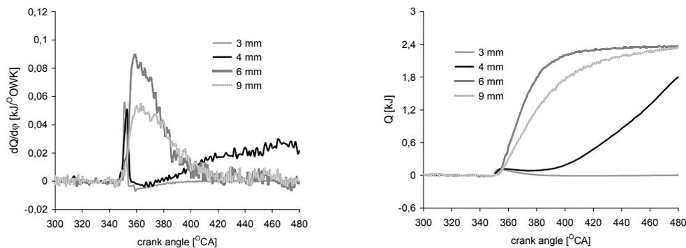
Fig. 14. Heat release rate and amount of heat released during combustion in function of CA for  $\lambda=2.0$
