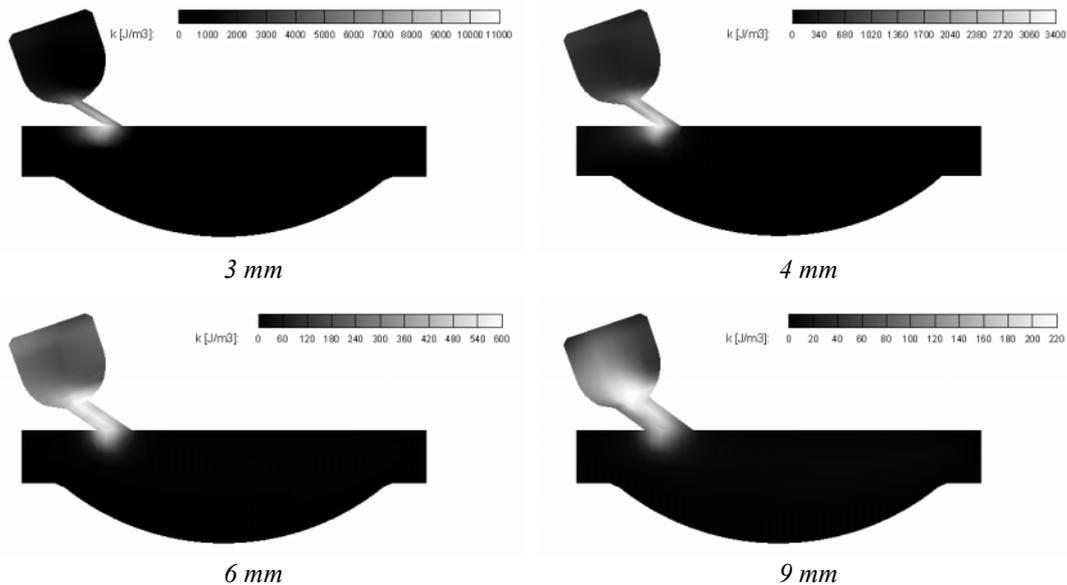
Fig. 5. The kinetic energy of turbulence distribution in combustion chambers of engine equipped with prechamber at the moment of spark discharge  $12^\circ\text{CA}$  before TDC
