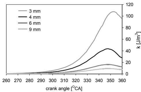
Fig. 3. The kinetic energy of turbulence averaged for both the cylinder and the prechamber of two-stage combustion system engine
