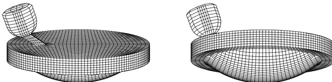
Fig. 1. Geometric mesh of combustion chambers at TDC
